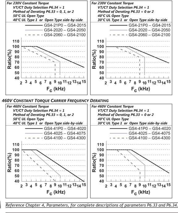
When working with P6.33 (Drive Derating Method), and P6.34 (VT/CT Duty Selection), refer to P2.10 (PWM Carrier Frequency) for the carrier frequency setting. When P6.34 is set it will change P2.10, while P6.00/P6.02 (Electronic Thermal Overload Relay (Motor1)/(Motor2)) must be set independently.
