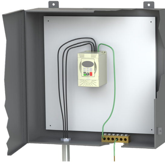
GS2 Input Wiring Routing
