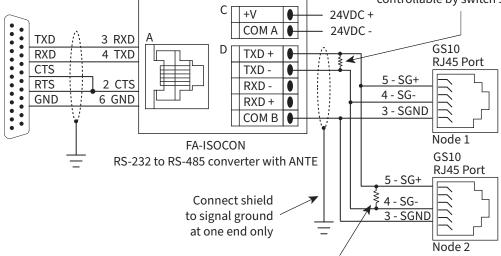
120Ω Termination Resistor at both ends of network
