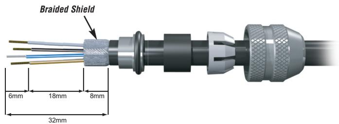
Strip wires and cut to the lengths shown to ensure a good fit when the connector is assembled.
