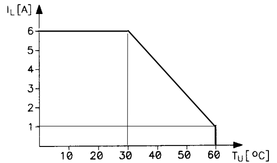
Derating curve Deratingkurve
