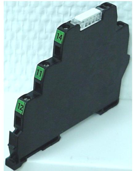
*The relay interface is used to suit various signal levels and to separate those galvanic. The control voltage is connected to terminal +A1, -A2. When applying the voltage the relay outputs switch over and die LED lights up.
