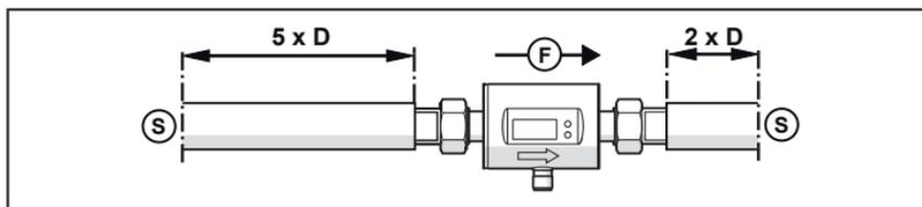
S = disturbance (e.g. shut-off / control device, pump, bends)
