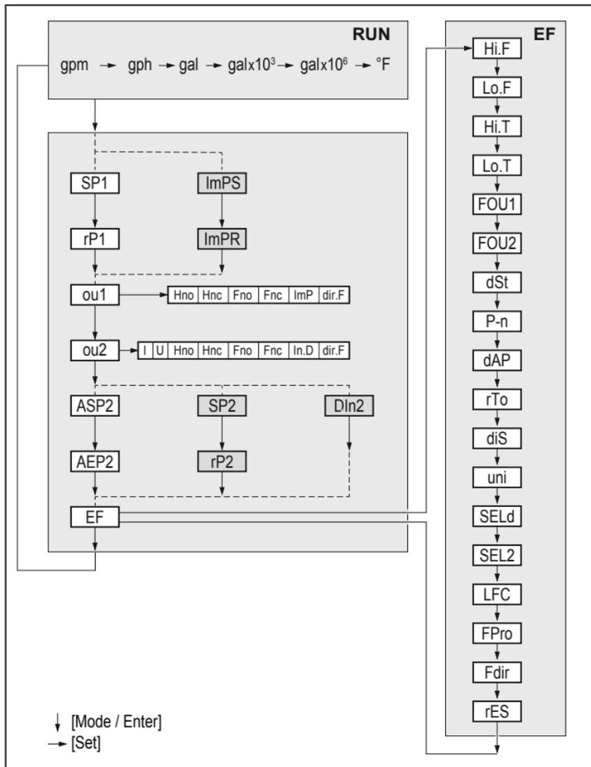
Parameters with white background are indicated in case of factory setting (→ 14). Parameters with grey background are indicated in case of changes of the preset for `ou1` and `ou2`.
