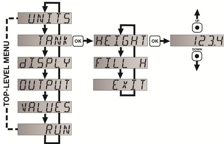
**Note:** The Height (4mA) and Fill Height (20mA) settings also determine the 4 to 20 mA current span.
