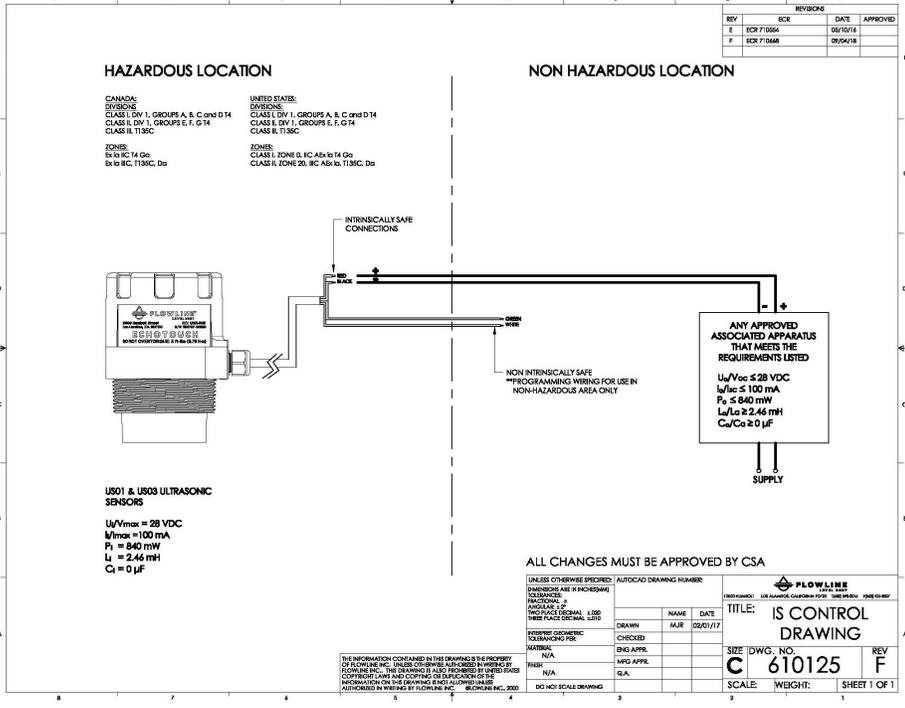
The cabling should be a shielded twisted pair to minimize EMI interference. Typically 20 to 24 gauge wire is used in this application.
