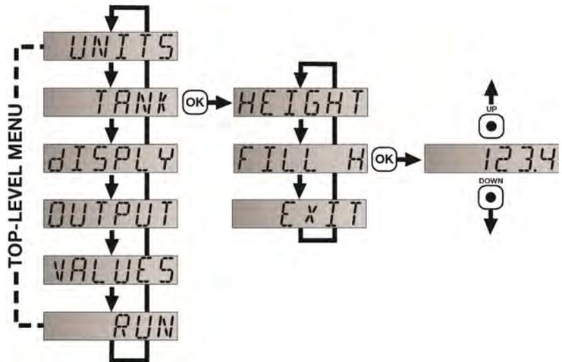
**Note:** The Fill-Height (**FILL-H**) setting determines the 20 mA current span. To reverse the current output with 4mA being at the top of the tank, use the **REV MA** function.
