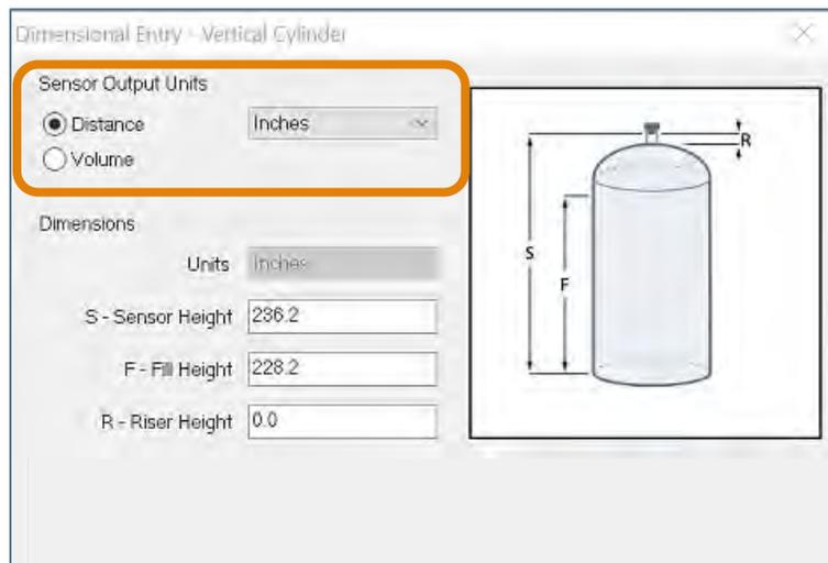
**Volume – Sensor Output Units (Vertical Cylinder Example):**
