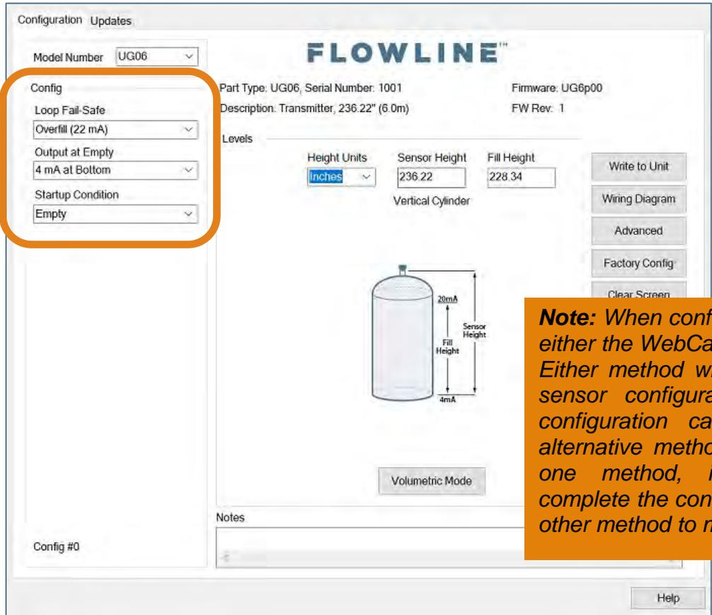
**Note:** When configuring EchoPod®, choose either the WebCal® or Push Button method. Either method will accomplish the goal of sensor configuration. Changes to the configuration can be made using the alternative method. When beginning with one method, it is recommended to complete the configuration before using the other method to make any adjustments.
