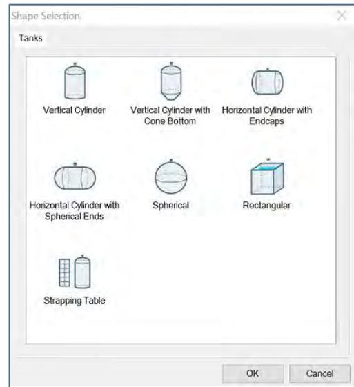
**A. Dimensional Entry – Vertical Cylinder Example:** Choose the Sensor Output Units as Distance or Volume. After choosing the Sensor Output Units, select the units of measurement in the pull down to the left.
