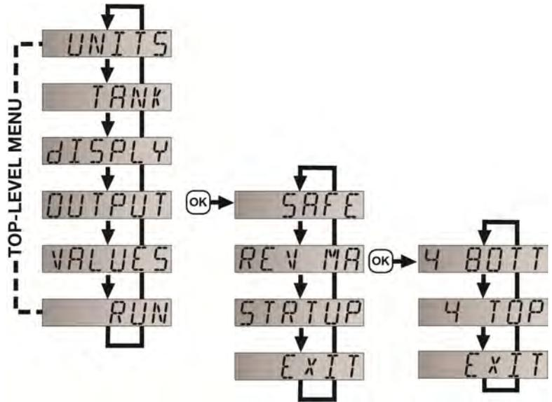
**HOW TO SETUP THE START-UP POWER (STRTUP)**
