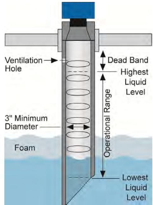
**Note:** Never allow the bottom of the stand pipe to become exposed to air. This will break the liquid seal which will prevent echoes from returning back to the sensor.
