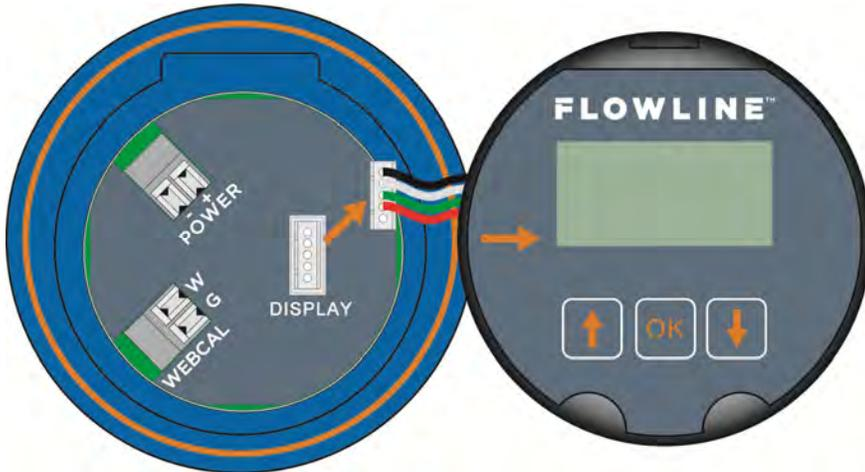
When wiring is completed, restore the display to the housing and replace the cover.
