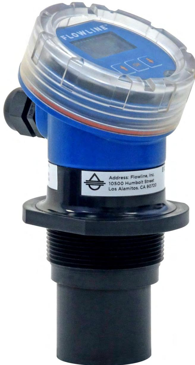
An ultrasonic sound wave is pulsed from the base of the transducer. The sound wave reflects against the process medium below it. The sound wave energy is returned to the transducer. The microprocessor based electronics measures the time of flight between the sound pulse generation and its receipt. This translates into the distance or range between the transducer and process media below.
