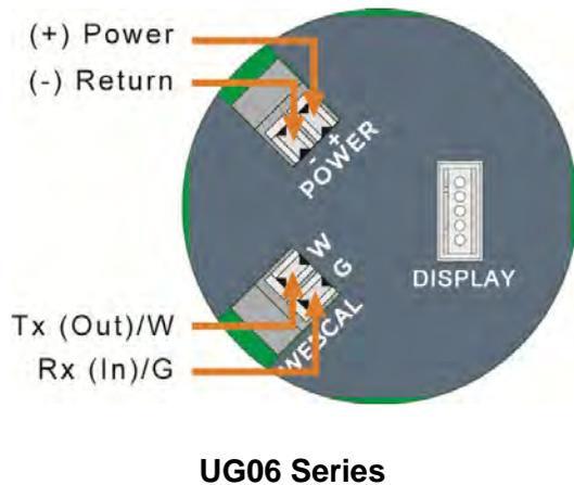
**(+) Power & (-) Return:** (+) Power and (-) Return leads are for connection to a 24 VDC power supply or to a 4-20 mA loop power source. The (+) and (-) wires can be extended up to 1,000 feet using a 22-gauge or larger wire.
