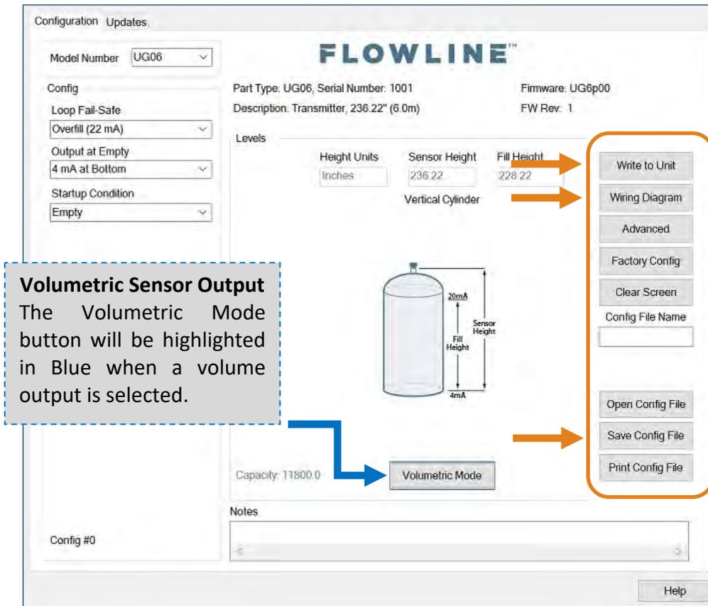
**Volumetric Sensor Output**
