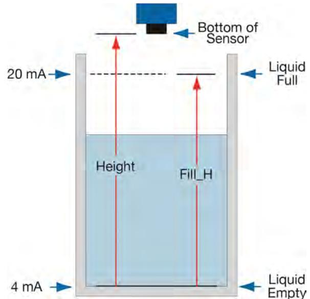
**Note:** The **HEIGHT** and Fill-Height (**FILL-H**) settings also determine the 4 to 20 mA current span. The **HEIGHT** setting determines the 4mA position and the **FILL-H** setting determines the 20 mA position.
