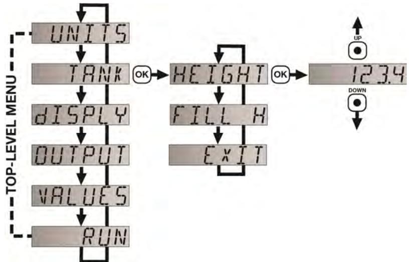
**Note:** The **HEIGHT** setting also determines the 4 mA current location. To reverse the current output with 20mA at the bottom of the tank, use the **REV MA** function.
