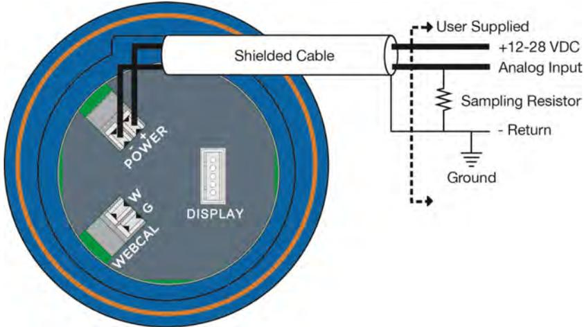
The cabling should be a shielded twisted pair to minimize EMI interference. Typically 20 to 24 gauge wire is used in this application. To access the terminals, gently remove the display from the housing.
