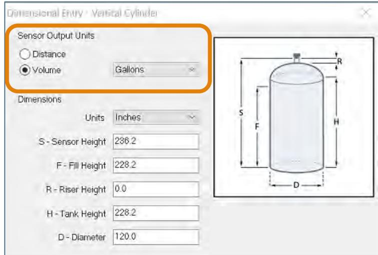
**Volume – Tank Capacity (Vertical Cylinder Example):** After entering the dimensions, press the Capacity button to show the Calculated Capacity of the tank. If the Calculated Capacity is slightly different than the expected capacity, click on the Adjust Capacity box and enter the expected capacity of the tank. If the Adjusted Capacity is more than 10% of the Calculated Capacity, recheck the dimensions information entered above.
