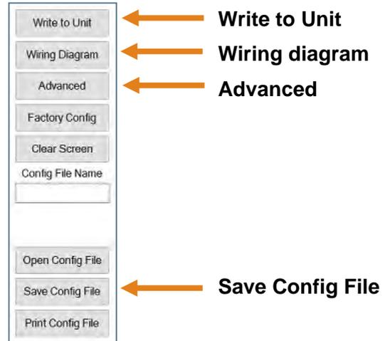
**“Save Config File”** will save this configuration as a text file which can be loaded back into WebCal® by pressing the **“Open Config File”** button. It is good practice to save the configuration file for each different configuration with a unique name for easy identification. If using multiple sensors in identical applications, then use of a single configuration file is recommended.
