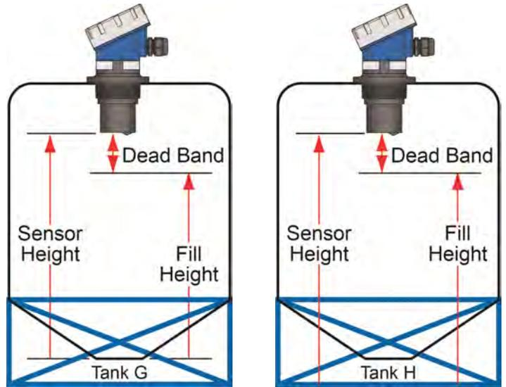
**Cone and Rounded Bottom Tanks**
