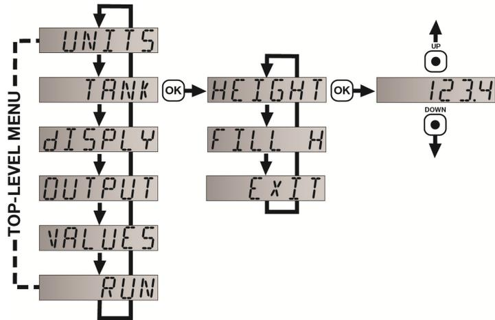
**Note:** The Height and Fill Height settings also determine the 4 to 20 mA current span. The Height setting determines the 4mA position and the Fill-H setting determines the 20 mA position.
