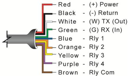
**Red & Black:** Red (Power) and Black (Return) leads are for connection to a 24 VDC power supply or to a 4-20 mA loop power source. The Red and Black wires can be extended up to 1,000 feet using a 22-gauge or larger wire; however do not extend the green and white wires beyond 15'.
