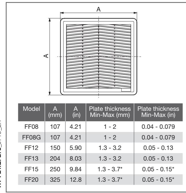
\* up to 4mm (0.16 in) with cut-out max tollerance.
