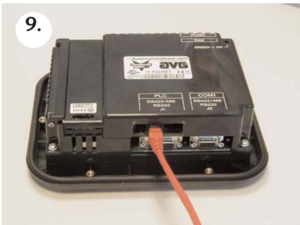
Close the back cover and press so it snaps back into place. Connect the ethernet cable as shown.
