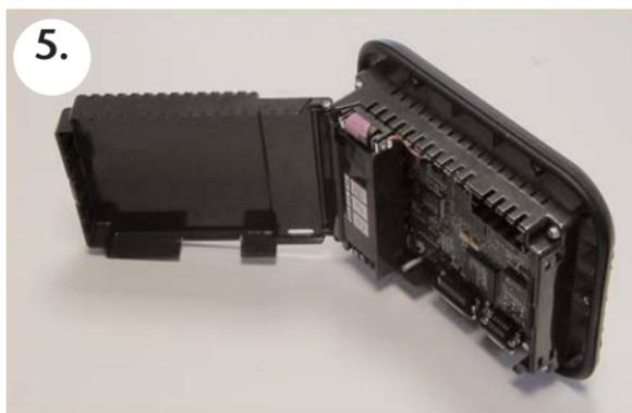
The EZ-Ethernet Card is now ready to be installed inside the EZTouch Panel.
