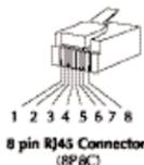
All Ethernet and ECOM patch cables should be Category 5, UTP Cable. The diagram illustrates the appropriate wire position in the RJ45 connector.
