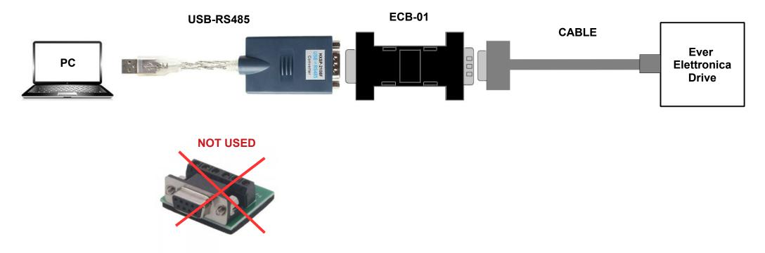
This is the only way to connect the Service KIT between drive and PC. Do NOT connect directly the USB-RS485 to the drive with cable, because this could cause damage the drive, PC or converter.
