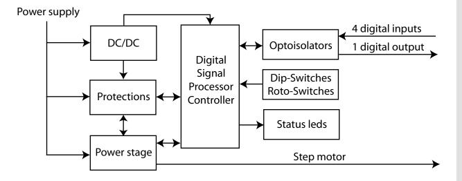
As shown in the block diagram, the functions of the drives are controlled by 4 digital opto-isolated inputs.
