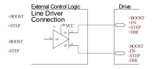
N.B. It's recommended to use 2Vdc digital inputs only in Line-Driver configuration to have more noise immunity..
