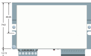
CN2: Digital inputs and output 10 position, pitch 3.81mm, PCB header connector
