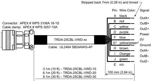
Connections for TRDA-25RNxxx-VWD-MS Line Driver Encoders and for Marathon Black Max Motors Dynapar HS35 Encoders
