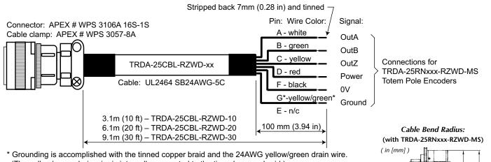
(The yellow/green drain wire is internally connected to the tinned copper braid.)
