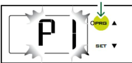
1. Press "PRG" button for 5 seconds to reach the modifiable parameter list.
