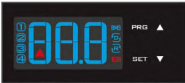
The display shows the temperature in the range of -50°C to +150°C (-58°F to +302°F). The temperature is displayed with resolution of tenths between -19.9°C and +99.9°C (-3.8°F to +211.8°F). During programming, it shows the codes and values of the parameters. The display also shows icons according to occurring events.
