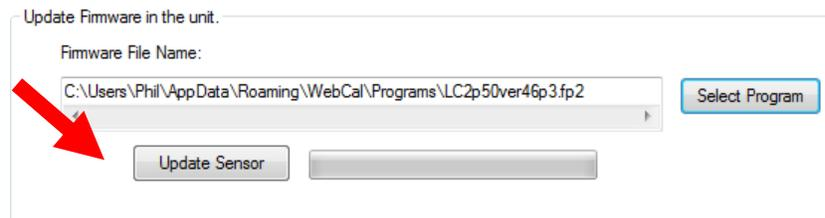
Confirm that the address is correct and then click on **Update Sensor** to begin the firmware update. This step should take less than 1 minute. You can follow the progress with the status bar to the right of the Update Sensor button. When completed, click on the Configuration tab to configure the transmitter. *Remember, when the firmware has been updated, the unit will return to its original factory settings.*
