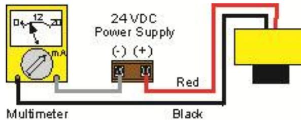
1. Connect a multimeter in series with the black wire to read the current output.
