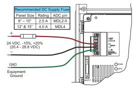
Recommended DC Power Supply: AutomationDirect Part No. PS24-050D
