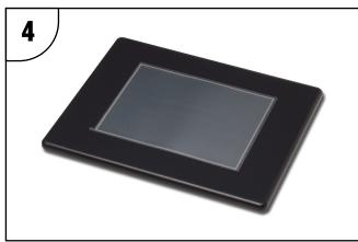
Smooth out the screen cover and press all around the outside perimeter to secure the cover in place. The screen cover can be removed by lifting up on the small tab and gently pulling the cover away form the touch panel's surface.
