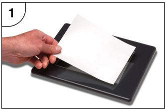
Check to be sure that the proper size non-glare screen cover is being used on the subject touch panel. Notice that the outer perimeter of the screen cover has an adhesive band. The adhesive band will be located on the outside edge of the touch panel's white frame bordering the touch area when installed.
