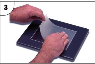
Align the screen cover over the touch panel's white frame, then start on one side and gently lay the cover over the entire touch area.
