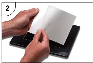
Start in one corner and peel the screen cover from the backing.
