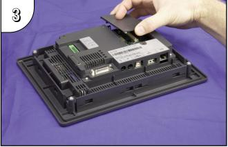
The cover will stop at the "Remove" position indicated by a tic mark on the cover lining up with the "Remove" tic mark on the panel. At this position, lift the cover up.
