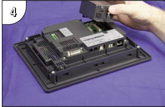
Position the expansion assembly over the opening so that the tic mark to the right of the fastening screw lines up with the "Remove" tic mark.
