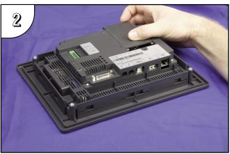
Remove expansion area cover by pressing down on the left and right line markings and at the same time, slide the cover in the direction of the embossed arrow.
