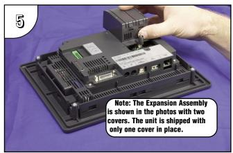
Slide the expansion assembly in a downward direction until the tic marks at the home position line up.
