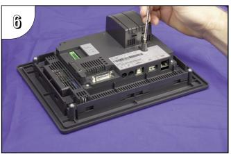
Secure the Expansion Assembly to the touch panel by tightening the spring loaded captive M3-20 screw to a torque of 50 oz-in [0.35 Nm].
