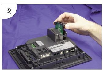
Install the CF Card Interface Module, p/n EA-CF-IF, into the right hand side slot by carefully aligning the female connector of the interface module with the male connector on the touch panel. There is guide at the top of the slot to accept the edge of the Interface Module's printed circuit board and another guide at the bottom to accept the edge of the plastic cover. It is also helpful to preset the locking tabs of the Interface Module so they are swung inward, top and bottom.
