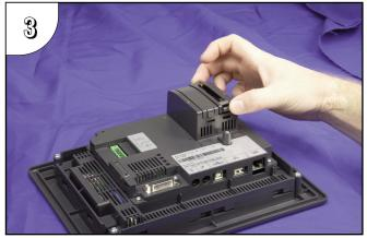
Continue to slide the interface module into the slot until the front of the module is flush with the front of the Expansion Assembly. Press on the front of the Interface Module until the locking tabs snap into place.
