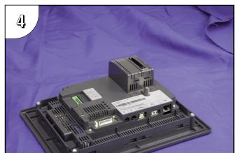
The above photo shows the CF Card Interface Module fully installed. To remove the Interface Module in the future, pry out on the top and bottom locking tabs at the same time and the module will release from the connector. Lift the module from the slot. The Interface Module should only be removed from the slot with input power disconnected.
