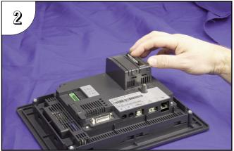
Gently press the CF card into the slot until it stops. You should feel a slight resistance as the CF card connector mates with the slot's connector. The CF card should be flush with the slot's opening.
