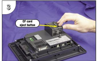
To remove the CF card from the CF Slot #2, press in on the eject button at the bottom of the CF card. This will cause the CF card to be partially ejected from the slot allowing removal.
