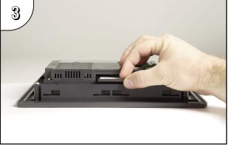
Orientate the compact flash memory card so that the front label is facing the back of the panel and the CF card connector faces into the slot. There are guides on each side of the slot that will match the guides on the CF card. The CF card can only be inserted one way.
