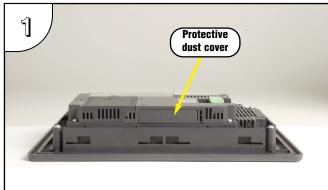
Remove the protective dust cover from the CF Slot #1 at the top of the touch panel by prying up on one edge. Sit the dust cover aside for re-installing after the CF card is installed.
