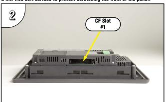
CF Slot #1 shown above with the protective dust cover removed.
