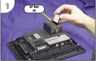
Orientate the compact flash memory card so that the front label is facing the power supply connector and the CF card connector faces into the slot. There are guides on each side of the slot that will match the guides on the CF card. The CF card can only be inserted one way.
