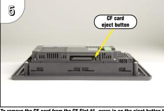
To remove the CF card from the CF Slot #1, press in on the eject button to the right of the CF card. This will cause the CF card to be partially ejected from the slot allowing removal.
