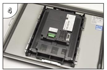
The above photo shows all mounting clips in place and the touch panel secured. The 8", 10" and 12" touch panels require 6 mounting clips and the 15" touch panel requires 8 mounting clips.
