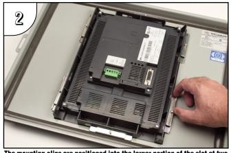
The mounting clips are positioned into the larger portion of the slot at two locations, and then slid torward the smaller protion of the slots to lock them in place. Some slots are arranged to slide to the left and others to the right.
