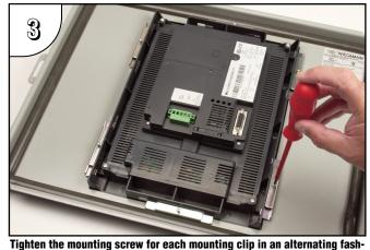
ion at all clips while observing the front of the touch panel. The goal is to make sure the front bezel is pulled up against the enclosure sheet metal uniformly, and the touch panel gasket is fully compressed all the way around its perimeter. Tighten the screws to a torque rating shown in the table below. Avoid over-tightening the screws to the point that they start to deform or bend the mounting clip.
