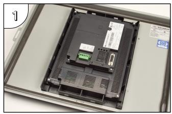
Position the touch panel through the cutout in the control cabinet door and hold in place. The mounting clips are postioned into the slots around the outside edge of the touch panel rear.
