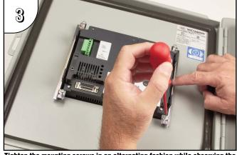
Tighten the mounting screws in an alternating fashion while observing the front of the touch panel. The goal is to make sure the front bezel is pulled up against the enclosure sheet metal uniformly, and the touch panel gasket is fully compressed all the way around its perimeter. Tighten the screws to a torque rating shown in the table below. Avoid over-tightening the screws to the point that they start to deform or bend the mounting clip.
