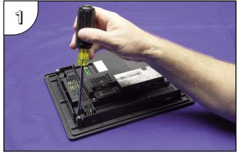
With power disconnected, use a #2 Phillips screwdriver to remove the four outer screws holding the touch panel's main electronics housing to the front bezel.
