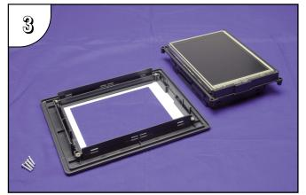
Place the new bezel facing down on the lint-free soft surface along with main electronics and four screws.
