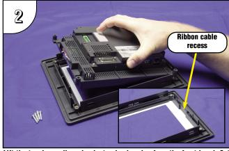
Lift the touch panel's main electronics housing from the front bezel. Set the four screws to the side and discard the original bezel. Observe the ribbon cable recess on the front bezel (see detail) for use in re-assembling the panel.
