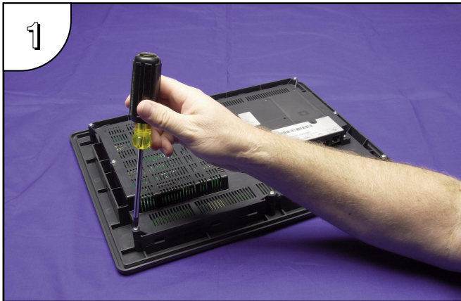
1 With power disconnected, use a #2 Phillips screwdriver to remove the eight outer screws holding the touch panel's main electronics housing to the front bezel.
