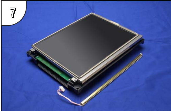
7 This photo shows the backlight bulb completely removed from its guide in the panel's main electronics housing.
