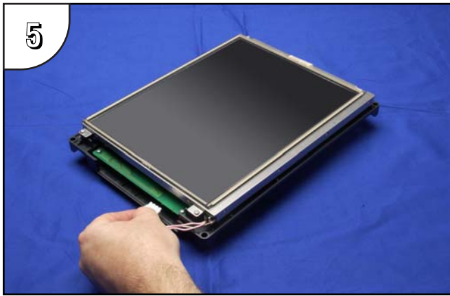
5 Unplug the backlight bulb's power cable connector from the circuit board connector.
