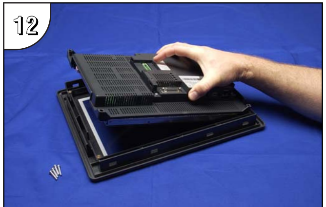
12 Position the touch panel's main electronics housing into the front bezel so that the flat ribbon cable on the housing aligns with the recess in the front bezel. Insert the four screws and tighten to a maximum of 70 oz-in [0.5 Nm].
