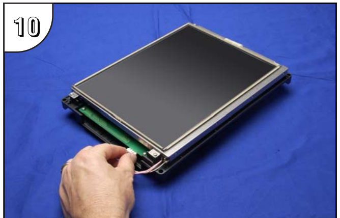
10 Plug the backlight bulb's power cable connector back into its circuit board connector.
