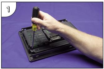
With power disconnected, use a #2 Phillips screwdriver to remove the four outer screws holding the touch panel's main electronics housing to the front bezel.
