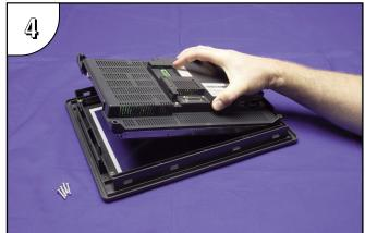
Position the touch panel's main electronics housing into the new bezel so that the flat ribbon cable on the housing matches up with the recess in the front bezel. Insert the four screws and tighten to a maximum of 70 oz-in [0.5 Nm].
