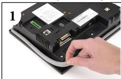
Start at one corner and pull the old gasket out of the channel that holds the gasket in place. Pull the gasket up as you work around the entire perimeter of the touch panel. Discard the old gasket.
