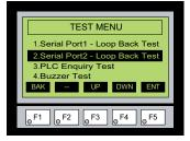
Serial Port 1 - Performs a test to verify the RJ12 serial communications port (Port 1) on the panel is operating correctly. Requires a loop back connector inserted into the port to properly run the test. A wiring diagram for the loop back connector is shown below.
