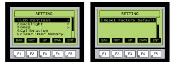
LCD Contrast - Used to adjust the LCD display's contrast. The default is a value of 3, and the range is 1 to 5, with 5 being the highest contrast.
