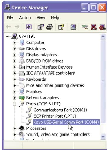
COM4 is the USB port used in this example. If you cannot find the **Koyo USB-Serial Comm Port** under Ports (COM & LPT) in **Device Manager**, the USB driver may not be correctly installed or the driver has a problem. Disconnect the cable from the PC and follow these steps to re-install the driver:
