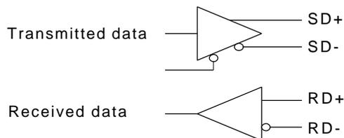
Note: A terminal resistor is not built in, so add one to the terminal board if necessary.
