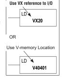
For example, you may want to read in a range of discrete input points to get a binary pattern into the CPU accumulator. The diagram shows two ways to reference the location.
