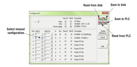
After the manual configuration has been set, save the configuration to the PLC and to the disk. The disk and PLC icon buttons located in the right-hand corner of the dialog allows the configuration to be either saved or read.
