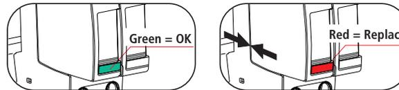
Fault Indication & Remote Contact Signaling (with modules installed)
