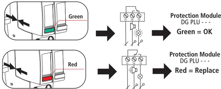
Testing Remote Contact Signaling (with modules installed)
