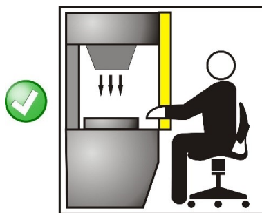
Figure 6: Correct light curtain positioning
