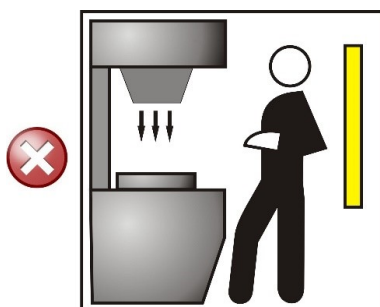
Figure 7: Wrong light curtain positioning
