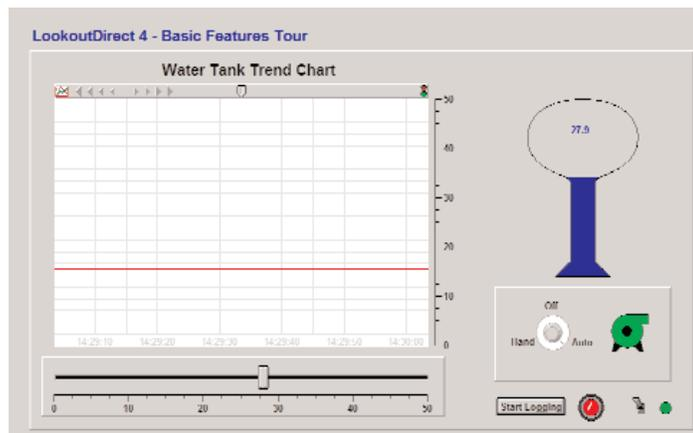
Click on the switch again and it will “flip” to the **OFF** position, turn off the new indicator and the EBC I/O point indicator will turn off.
