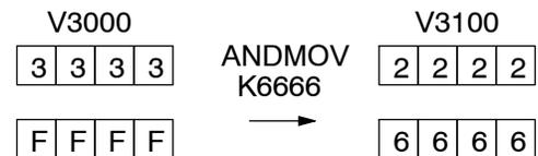
The program on the next page performs the ANDMOV operation example above. It assumes that the data in the table at V3000 - V3001 already exists. First we load the table length (two words) into the accumulator. Next we load the starting address of the source table, using the LDA instruction. Then we load the data into the accumulator to be ANDed with the table. In the ANDMOV command, we specify the table destination, V3100.
