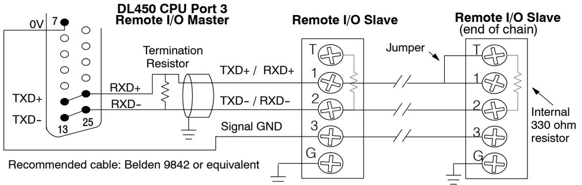
The twisted/shielded pair connects to the DL450 Port 3 as shown. Be sure to connect the cable shield wire to the signal ground connection. A termination resistor must be added externally to the CPU, as close as possible to the connector pins. Its purpose is to minimize electrical reflections that occur over long cables. Be sure to add the jumper at the last slave to connect the required internal termination resistor.
