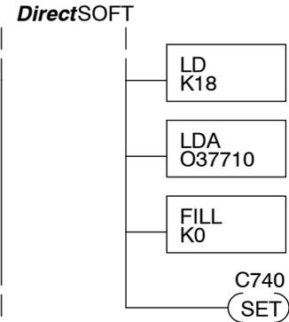
On the last rung in the example program above, we set a special relay contact C740. This particular contact indicates to the CPU that the ladder program has just finished specifying a remote I/O system. At that moment the CPU begins remote I/O communications. Be sure to include this contact after any Remote I/O setup program.
