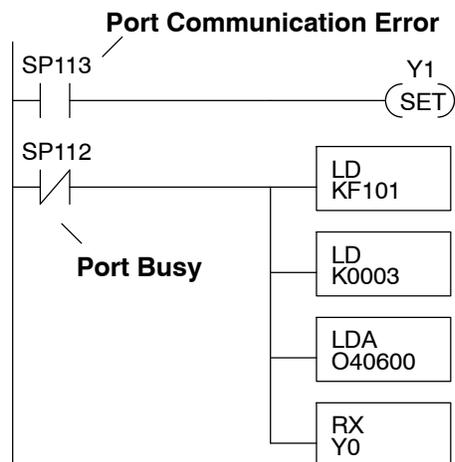
Each port which can be a master has two Special Relay contacts associated with it (see Appendix D for comm port special relays). One indicates “Port busy”, and the other indicates ”Port Communication Error”. The example above shows the use of these contacts for a network master that only reads a device (RX). The Port Busy contact ensures one network transaction finishes before we begin another.
