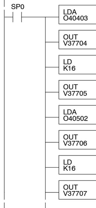
When configuring a Remote I/O channel for fewer than 7 slaves, we must fill the remainder of the table with zeros. This is necessary because the CPU will try to interpret any non-zero number as slave information.
