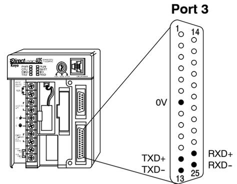
Now we are ready to discuss wiring the DL450 to the remote slaves on the remote base(s). The remote I/O link is a 3-wire, half-duplex type. Since Port 3 of the DL450 CPU is a 5-wire full duplex-capable port, we must jumper its transmit and receive lines together as shown below (converts it to 3-wire, half-duplex).
