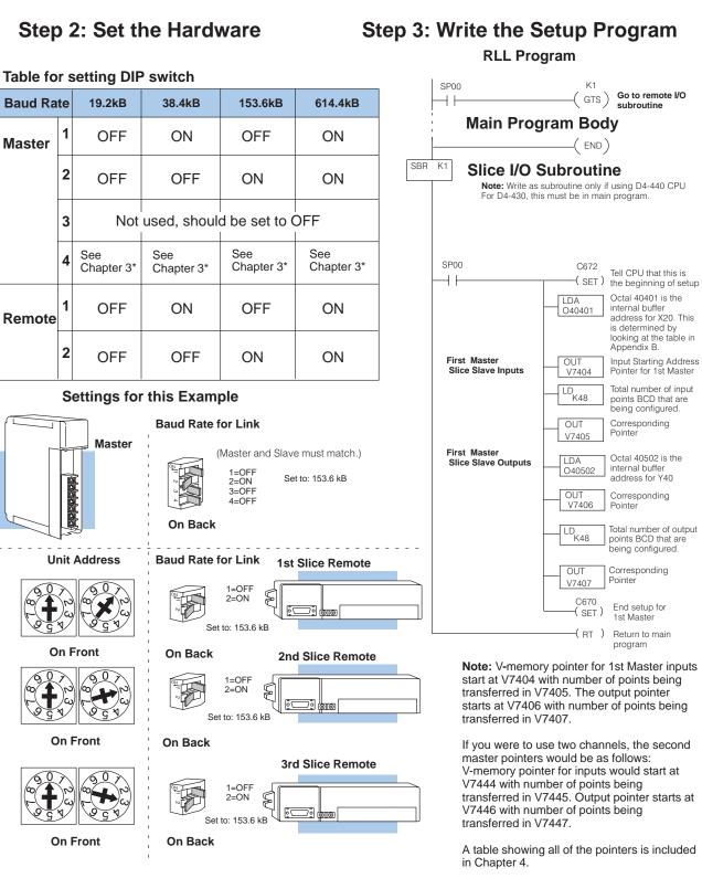
\*In Chapter 3, you will learn how the setting of the binary switch on the master module affects the system's ability to make use of discrete addressing and the system's slave removal process. C670 ends the setup for 1st Master, but C674 must end the setup for 2nd Master.
