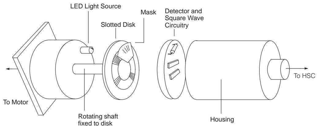
The quantity of slots on the disk is equivalent to the number of pulses per turn. Most quadrature encoders also provide a single isolated slot on the disk called the Z marker. It is aligned with its own separate LED. The pulse from this channel provides a reference once per revolution. The automatic home search function, built into the HSC, makes use of the Z-marker when you connect a quadrature encoder to the HSC with the Z-marker attached to **INZ**.
