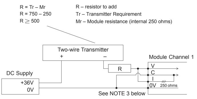
NOTE 3: When a differential input is not used, 0V should be connected to C of the channel.
