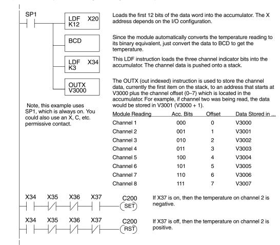
Scaling the Input Data The Thermocouple Input module automatically converts the temperature readings into the digital equivalent, so as long as you are using the module to monitor temperatures you never have to perform any scaling. However, there are two situations where you will probably want to understand how to scale the data.
