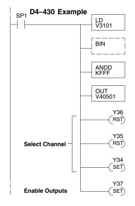
The LD instruction loads the data for channel 1 into the accumulator. Since SP1 is used, this rung automatically executes on every scan. You could also use an X, C, etc. permissive contact.
