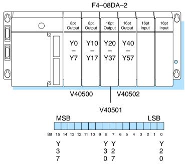
Within this V-memory location the individual bits represent specific information about the channel selected and the analog signal.
