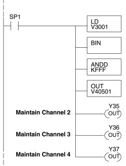
The LD instruction loads the data for channel 1 into the accumulator. Since SP1 is used, this rung automatically executes every scan. You could also use an X, C, etc. permissive contact.
