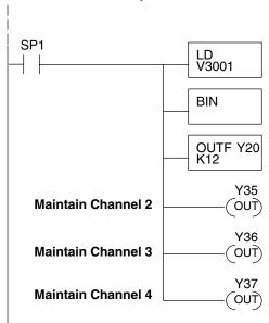
The LD instruction loads the data for channel 1 into the accumulator. Since SP1 is used, this rung automatically executes on every scan. You could also use an X, C, etc. permissive contact.
