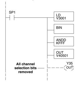
The LD instruction loads the data for channel 1 into the accumulator. Since SP1 is used, this rung automatically executes on every scan. You could also use an X, C, etc. permissive contact.
