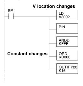
The LD instruction loads the data for channel 1 into the accumulator.
