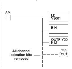
The LD instruction loads the data for channel 1 into the accumulator. Since SP1 is used, this rung automatically executes on every scan. You could also use an X, C, etc. permissive contact.
