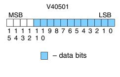
Since the module has 12-bit resolution, the analog signal is made of 4096 "pieces" ranging from 0 – 4095 ( $2^{12}$ ). For example, with a 0 to 10V scale, you would send a 0 to get a 0V signal, and 4095 to get a 10V signal. This is equivalent to a binary value of 0000 0000 0000 to 1111 1111 1111, or 000 to FFF hexadecimal. The following diagram shows how this relates to each signal range.
