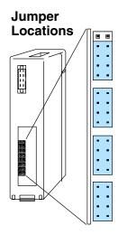
If you examine the rear of the module, you will notice several jumpers. These jumpers are used to select the signal range for each channel. There is also a current jumper. Some of the ranges can be selected with the current jumper installed or removed. To prevent losing jumpers when they are removed, a good place to store them is to reinstall each removed jumper over a single pin.
