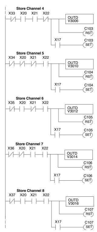
This rung looks at fault bit X33 (the broken transmitter bit for channel 4) ANDed with active channel bits X20–X22. When the active channel bits are true and there is no transmitter fault, channel 4 data is stored in V3006.
