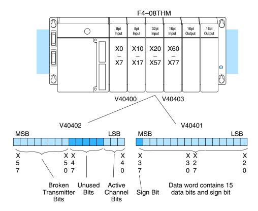
Analog Data and Sign Bits The first 16 bits represent the analog data in binary format. The MSB is the sign bit.
