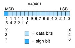
The active channel bits represent the channel selections in binary format (000 = channel 1 is active, 001 = channel 2 is active, 111 = channel 8 is active, etc.).
