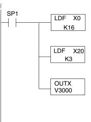
Note: This example uses SP1, which is always on. You could also use an X, C, etc. permissive contact. Loads the 16 bits of channel data (starting with location X0) from the module into the accumulator.
