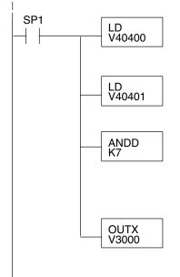
Loads all 16 bits of the channel data (first word) from the module into the lower 16 bits of the accumulator. This example assumes that the module location starts in the X0 position of the base.
