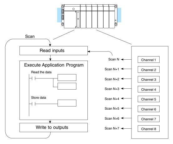
Even though the channel updates to the CPU are synchronous with the CPU scan, the module asynchronously monitors the thermocouple signal and converts the signal to a 16-bit binary representation. This enables the module to continuously provide accurate measurements without slowing down the discrete control logic in the RLL program.
