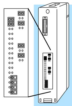
Step 3 . Connect the field wiring to the module connector.
