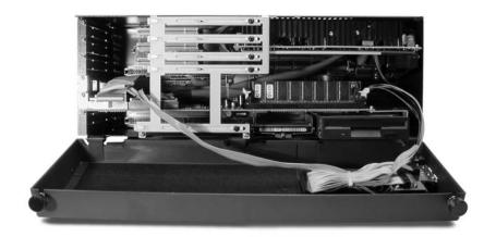
As you will notice in the photo below, we removed the backplane circuit board from the D4–470 case to facilitate veiwing. *Do not* remove the backplane board to install expansion boards.
